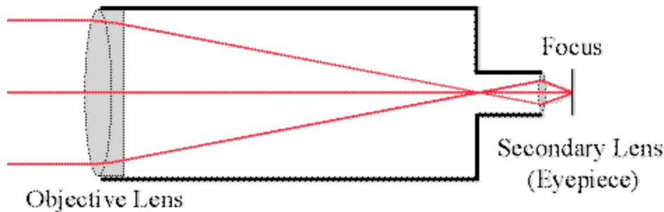
**Achromatic** – These were the first type of telescopes. They had chromatic aberration of the lens which shows itself as fringes of color around the image. This occurs because all colors cannot be focused at a single common position on the optical axis.
