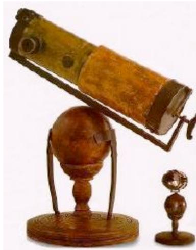
His selection of material to make the reflecting surface was an alloy of copper and tin. He polished and smoothed the mirror until he felt it overcame the aberrations caused by the refracting lenses. It actually took a while for his telescope to catch on but eventually as the technique was perfected the advantages of his design won over principally due to the much more manageable size and higher light gathering capability.
