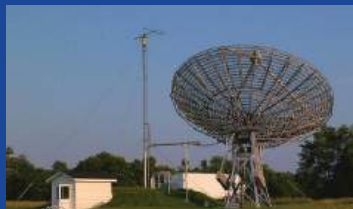
SARA members have been privileged to use this forty foot diameter drift-scan hydrogen line radio telescope every year at their annual meeting in Green Bank.
